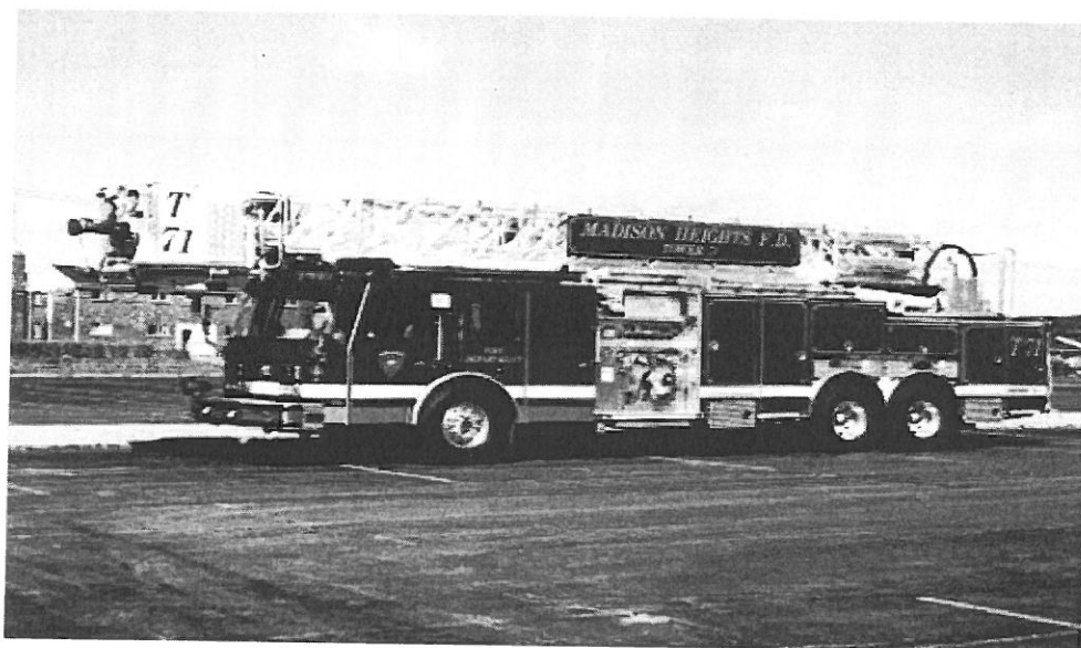
1998 E-One 95-foot Aerial Tower. This truck has a 1500 g.p.m. pump with 1500 g.p.m. cannon at the basket. This rig comes with a full compliment of ground ladders, 750 feet of 5-inch supply hose, 200 gallons of tank water and can be set up by one person in 2 minutes. This unit is housed at Station #1.
